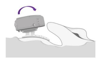
To attach the ADHEAR processor, you tilt the audio processor at a slight angle onto that snap connector.
